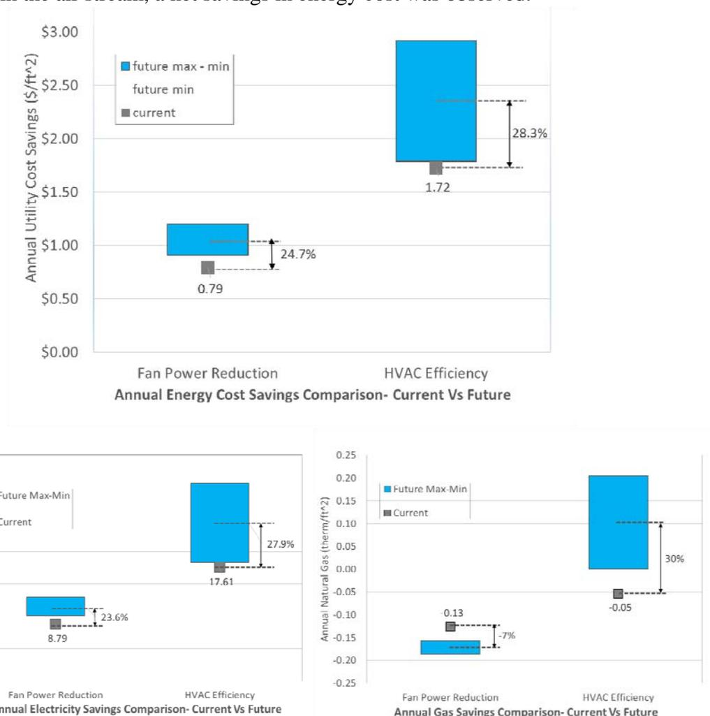
Figure 4: Annual cost and energy savings potential comparison under current and future climate scenarios for HVAC upgrades.
