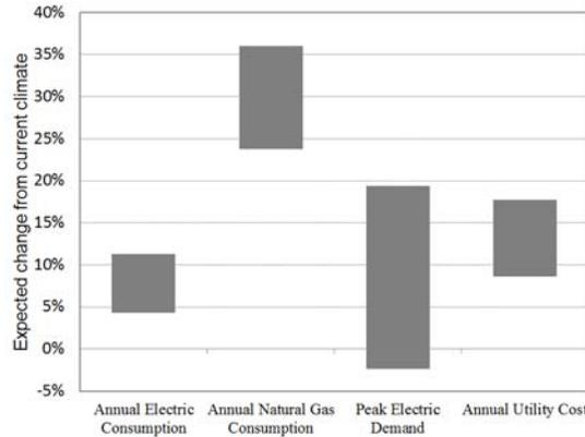
Figure 2: Expected change in building performance for each climate scenario at SSC.
