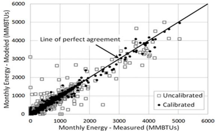
Figure 1: Monthly modeled versus measured energy usage for all existing models before and after calibration.
