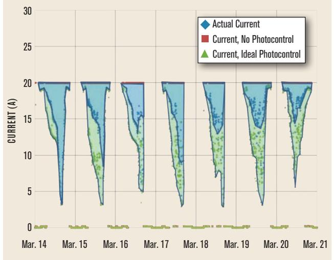
before commissioning and after. As in any multi-period energy study, we normalized all of these for weather effects (e.g., available daylight) between these periods, with the ultimate results representative of a Typical Meteorological Year.
