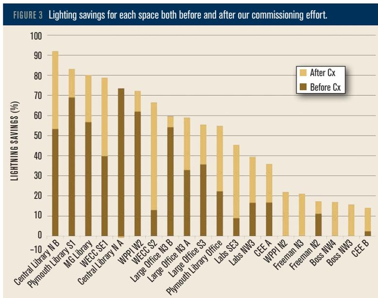
performance of the control itself. Initially, we found the average controls effectiveness in the as-found condition to be 51% (with a median of 66%). However, the spaces in our study displayed a wide range of performance. Four did not work at all, showing an effectiveness of zero. On the other end of our spectrum, over half of the spaces had effectivenesses of more than 60%.
